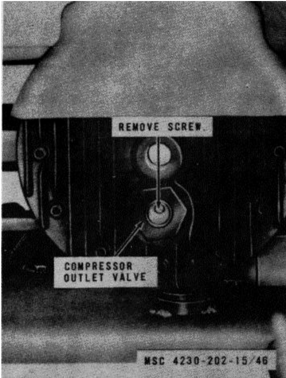
Figure 3-39. Compressor outlet valve, removal and installation
